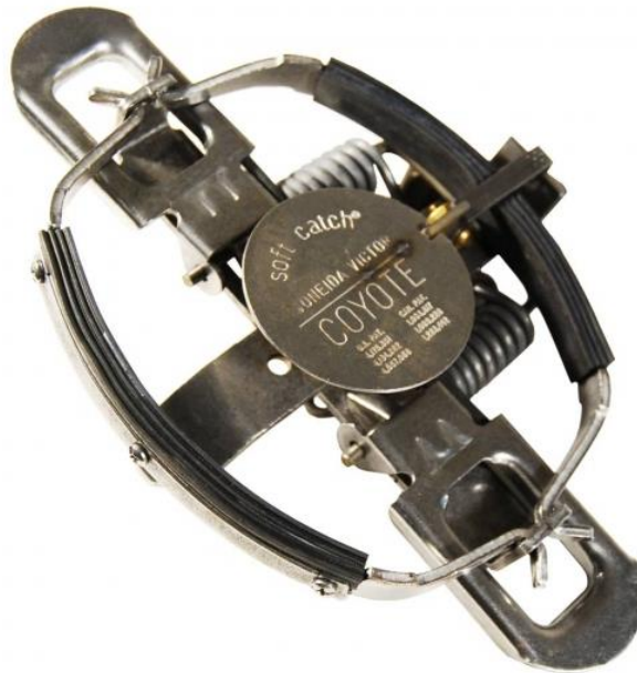
Photo 13. A leg-hold trap used for trapping pelicans. Notice that the jaws of the trap are covered in rubber to eliminate the risk of injury. Also, the trap is purposely manufactured with slightly off set jaws for a softer catch, the drawback being that the pelican has some chances of escaping if the leg is only partially caught (source: https://www.wildlifecontrolsupplies.com ).
